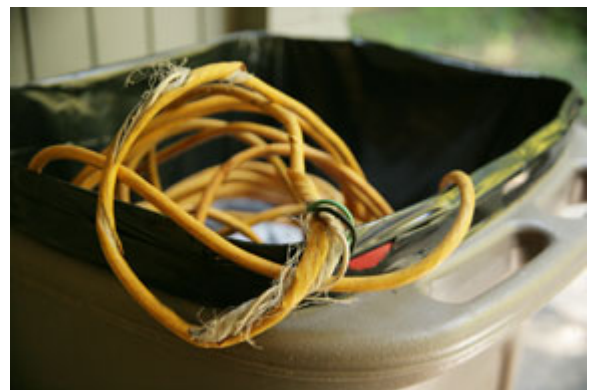
Replace worn, old, or damaged appliance cords right
